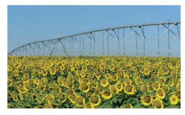
[LESA] and low energy precision application [LEPA] have been added to center pivot machines to apply water very close to or on the soil surface of the field to improve application efficiency.
