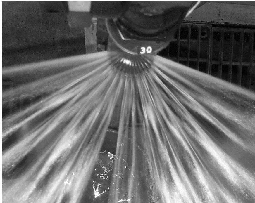
Figure 4:32 Test 5 – Sprinkler pattern
