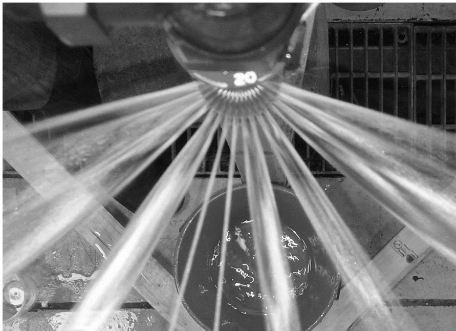
Figure 4:29 Test 4 – Sprinkler pattern
