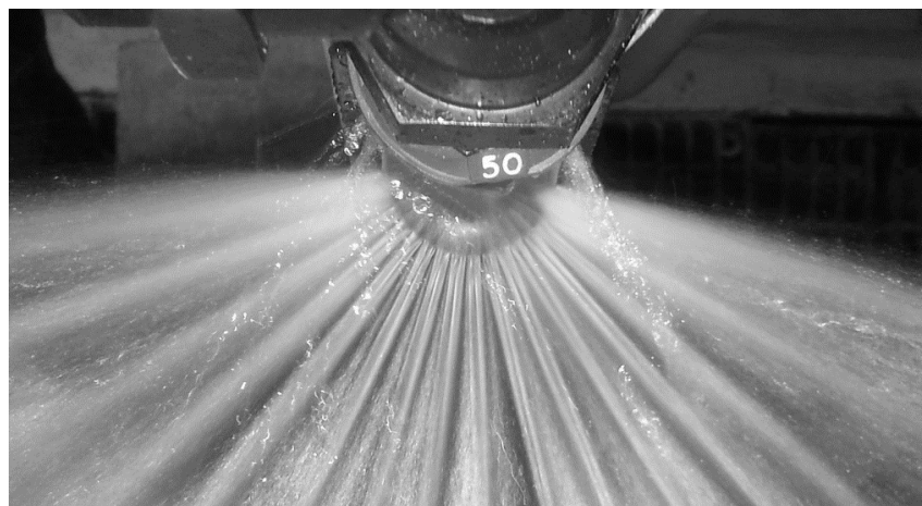
Figure 4:41 Test 8 – Sprinkler pattern
