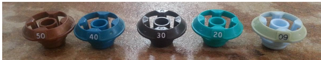
Figure 3:3 Nozzles used during the static plate test
