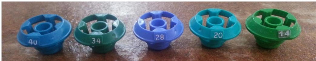
Figure 3:2 Nozzles used for the spinning plate tests
