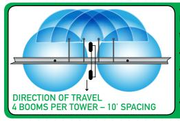
Installing PC-R3000 Rotators on Hose Booms minimizes wheel tracking issues and maximizes the effectiveness of part-circle devices as compared to mounting on straight drops. Featuring built-in dampening and directional control, the side force associated with part-circle sprinklers is absorbed for system stability and extended wear life. A typical application is to install 4 booms per tower with 10 foot spacing.
